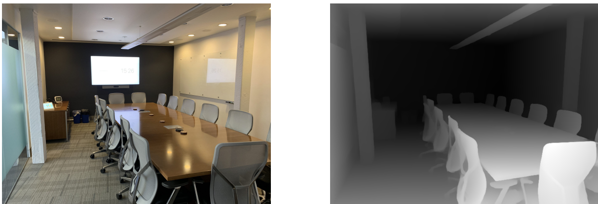
Figure 7.3: Output from the depth estimation model. Lighter regions indicate pixels estimated to be closer to the camera (at a smaller depth).
